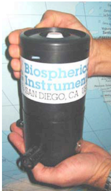
Figure A6: Aquatic BIC Radiometer with optional temperature and pressure sensors
