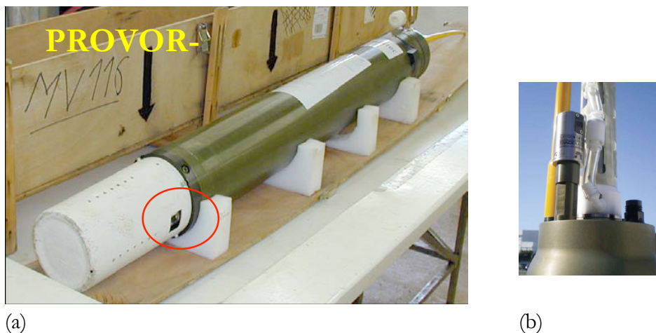
Figure 4: a) First model of PROVOR-DO, equipped with an Aandera optode at the bottom of the float; b) on recent PROVOR-CTS3-DO floats, the optode is located on top, near the CTD.
